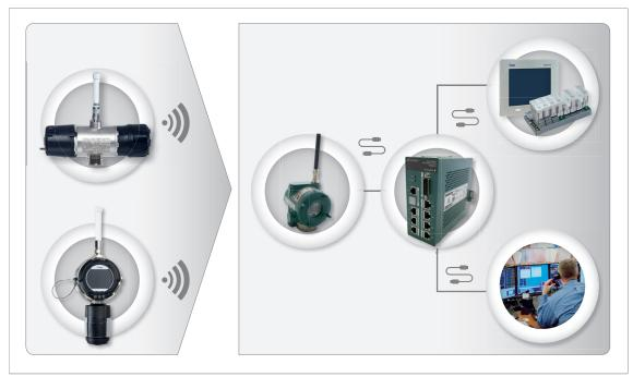
The wireless transmitters send their detection signal to the access point. From there, the signal is transferred to the gateway, which feeds the control unit directly via Modbus or using the PROFINET® protocol.
