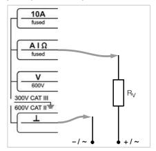
(without transient resistor!) in series with the power consumer  $\boldsymbol{R}_{\boldsymbol{v}}$  . With DC current note the polarity!
