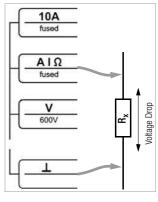
limit of the protective means is 200 A $\!\!\approx$  at a maximum (one half wave) on 600  $V_{\text{eff}}.$
