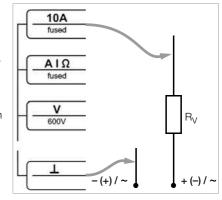
measuring leads (without transient resistor!) in series with the power consumer R<sub>v</sub>. With DC current note the polarity!
